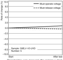
Characteristics were measured after applying a shock of  $490~\text{m/s}^2$  to the test piece 3 times each in 6 directions along 3 axes.
