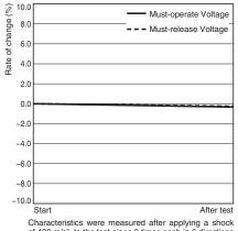
Characteristics were measured after applying a shock of 490 m/s $^2$  to the test piece 3 times each in 6 directions along 3 axes. The percentage rate of change is the average value for
